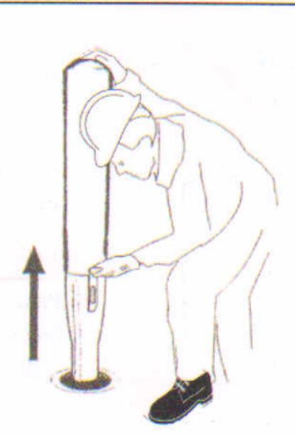
With key fully engaged , lift to remove bollard.
