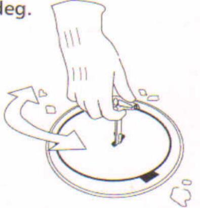
3. Lift blanking cap with key.
