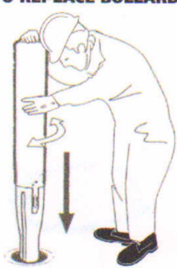
3. Insert bollard stem into sprocket and twist until bollard drops to engage.
